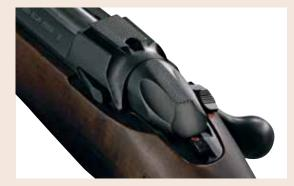
The lengthened rear bolt guide makes an already smooth action even smoother. Typically, the shorter the action the more susceptible it is to bolt bind due to decreased bearing surface area. The lengthened rear bolt guide surface of the Sako 85 ensures the smoothest possible bind-free bolt travel, even in the very popular WSM chamberings.
